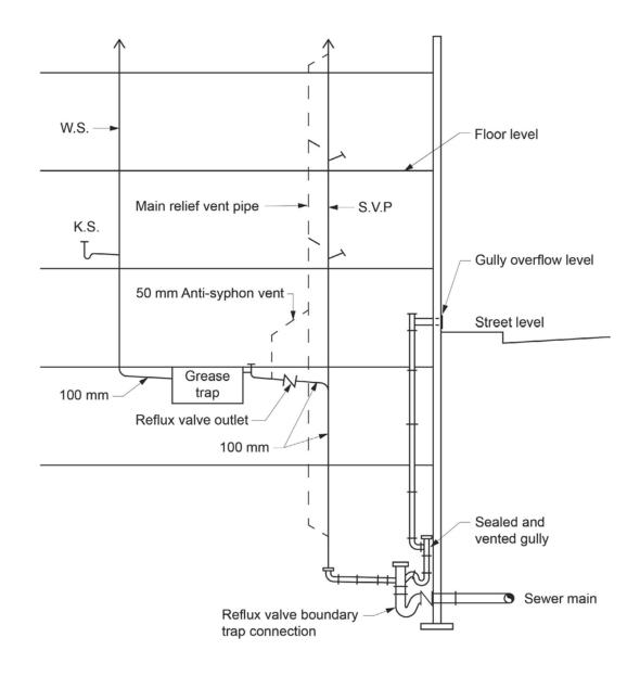
Tas Figure H202.4i Grease trap installation within multi-storey building
