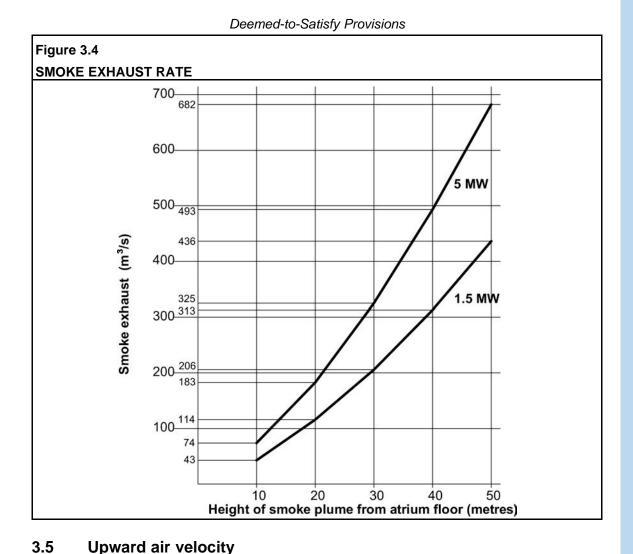
Notwithstanding **3.4(c)**, the average upward air velocity in the *atrium*, due to the *required* smoke exhaust quantity must—
