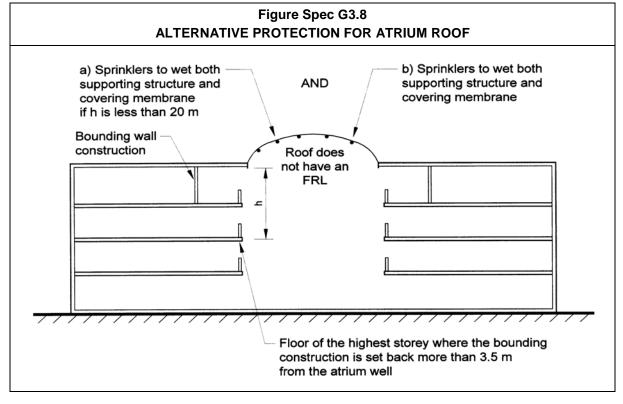
When the roof is required to have an FRL, **G3.6(a)** does not allow the use of the concessions contained in **Clauses 3.4, 3.5** or **3.6** of **Specification C1.1** for the roof of the atrium.
