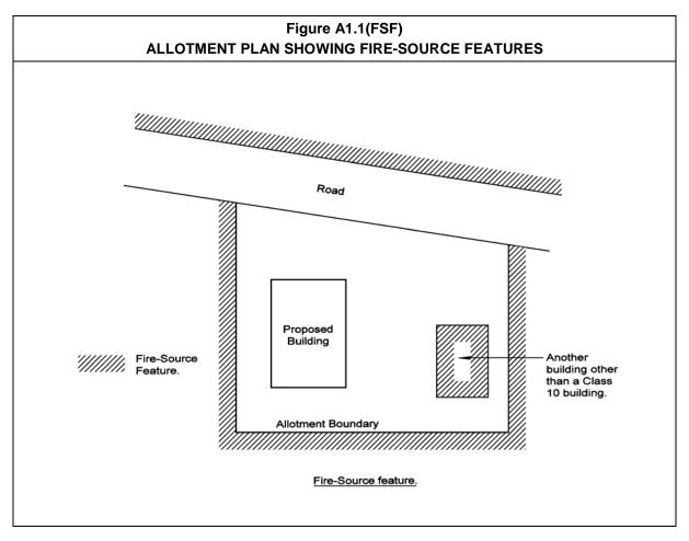
Note that the term 'fire-source feature' does not necessarily apply to a building - it relates to a potential source of fire. That potential may be realised in the future construction of a building. For this reason, the fire-source feature is not simply a line on the ground, nor a point at the top of a building; it is a continuous plane rising above that line or point.
