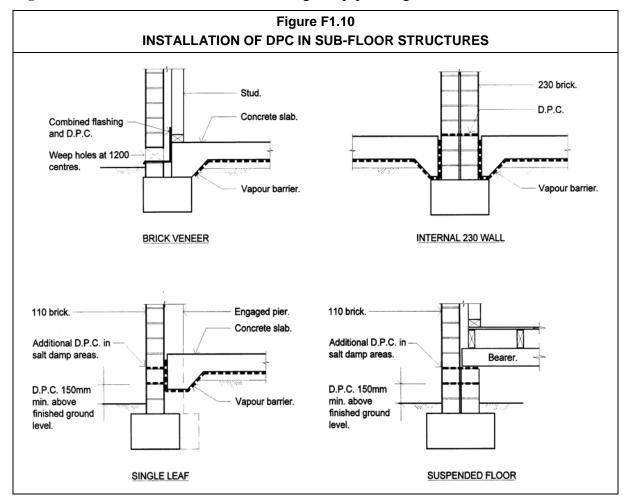
Figure F1.10 illustrates a method of installing damp-proofing in sub-floor structures.
