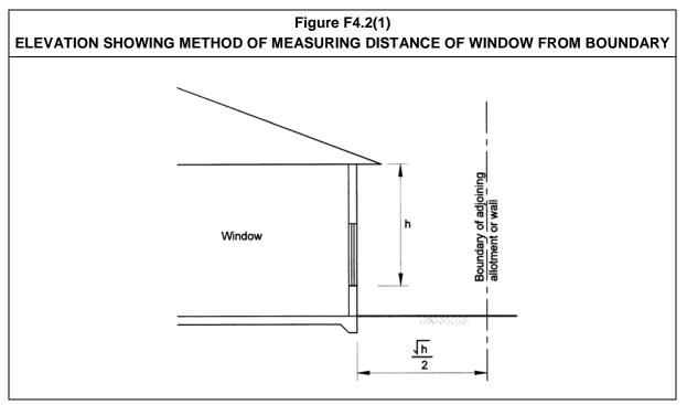
**F4.2(b)** does not prohibit windows closer to the boundary than one metre (or three metres in the case of a patient-care area in a Class 9a building). However, if a window is located within these distances, **F4.2(b)** does not allow it to be considered as providing required natural light to the subject room.
