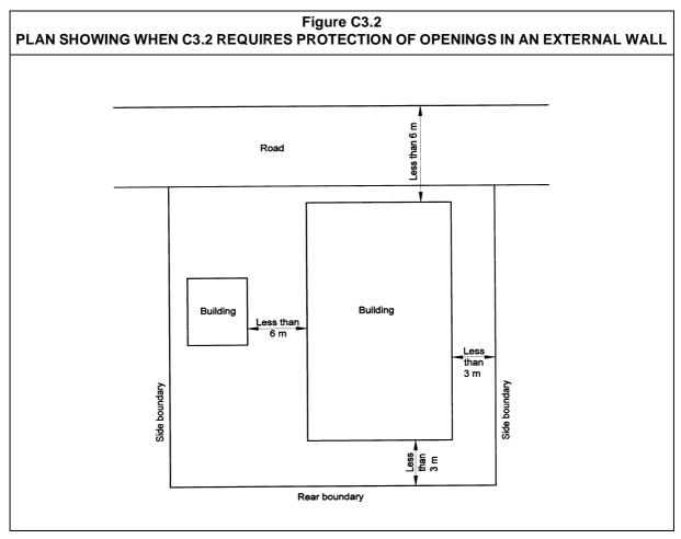
Under C3.2(c), openings in an external wall must be limited to the size specified, if the openings are required to be protected under C3.2(b). This is unless the openings are in a Class 9b open spectator stand.
