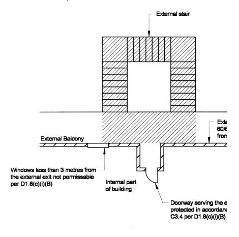
**D1.8(d)** provides requirements for the shielding construction and protection of any openings in that construction.
