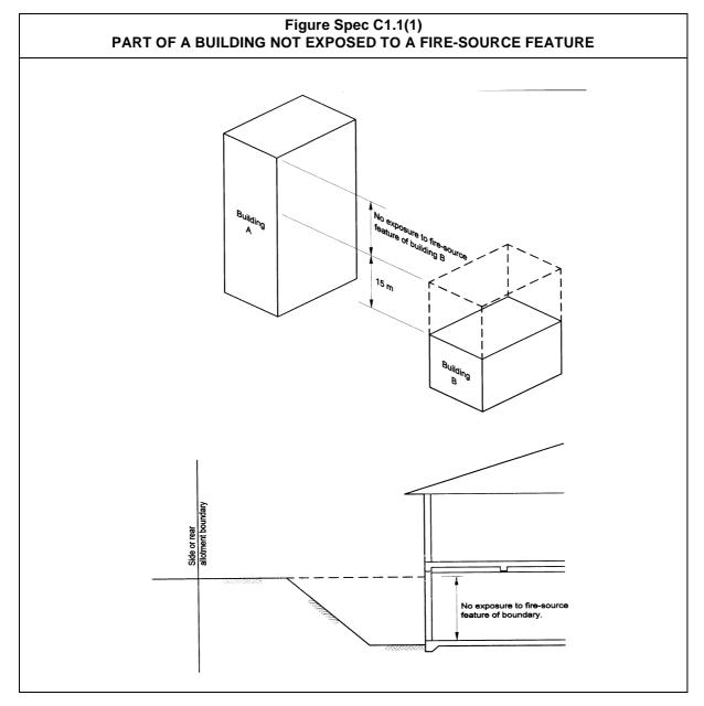
The building element must have an FRL required for the closest part of the element exposed to the fire-source feature (see Clause 2.1(c)(i)).
