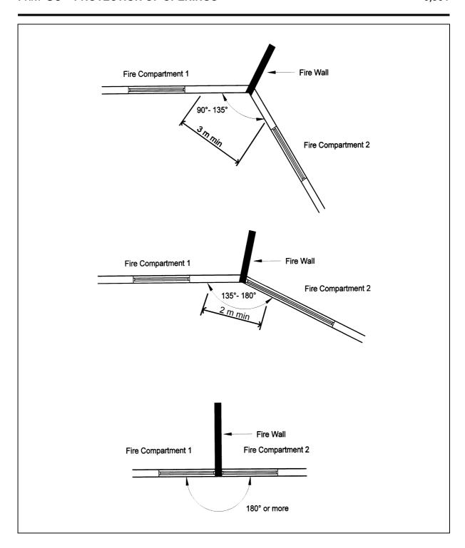
C3.3 only applies to external walls. It does not apply to fire walls separating fire compartments. (A fire wall is not always an internal wall. See Figure C2.7(3) of this Guide).
