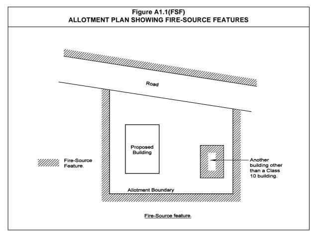
Note that the term 'fire-source feature' does not necessarily apply to a building - it relates to a potential source of fire. That potential may be realised in the future construction of a building. For this reason, the fire-source feature is not simply a line on the ground, nor a point at the top of a building; it is a continuous plane rising above that line or point.
