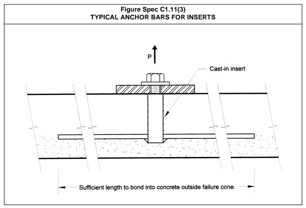
Clause 3(b) sets out the strength capacity required for top inserts or fixings so that the collapsing framework or roof structure will pull the panel inwards. See Figure Spec C1.11(4).
