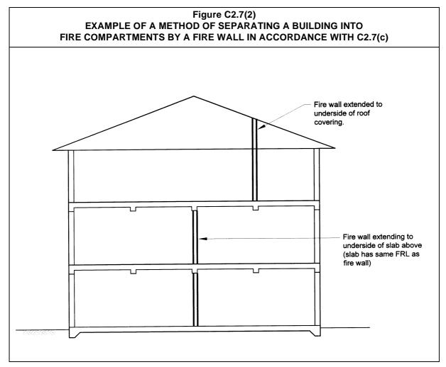
For a fire wall to compartment a building it must extend to the underside of any roof covering or between floors that have an equivalent FRL to the fire wall.
