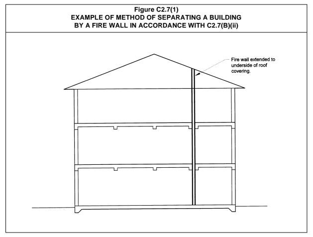
C2.7(a)(iii) indicates which building elements are permitted to pass through or cross a fire wall and prohibits the use of any building element if it reduces the fire wall's FRL below that required. Hence, elements that pass through or cross a fire wall have to be part of the fire wall's tested prototype.
