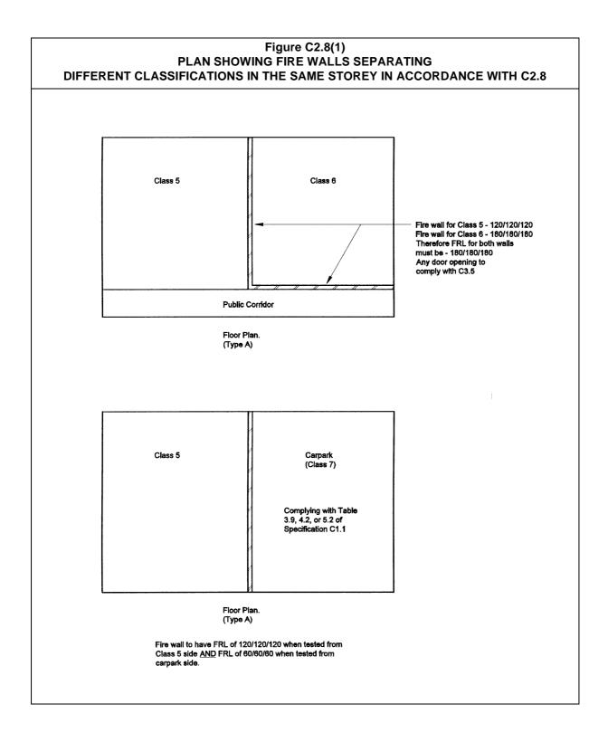
The diagrams in **Figure C2.8(2)** illustrate examples of fire walls separating different classifications within the same storey of a multi-storey building and floors separating different classifications.
