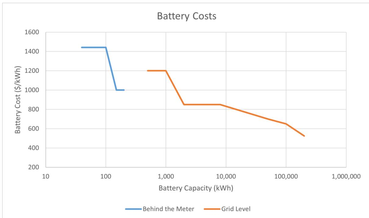
Figure 17: Battery Cost Behind the Meter and Grid Level Expressed as \$/kWh
