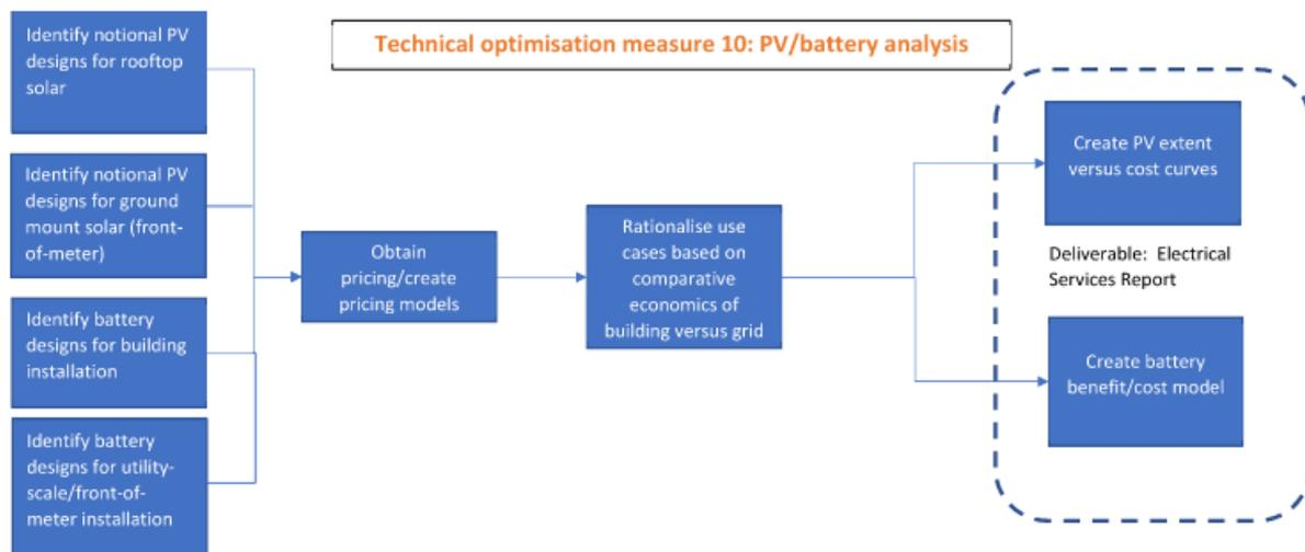
Figure 8. Outline methodology for the PV/Battery analysis
