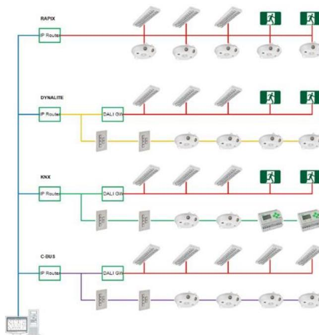
Figure 37: LCS-05 – Digital Addressable Lighting Interface (DALI)
