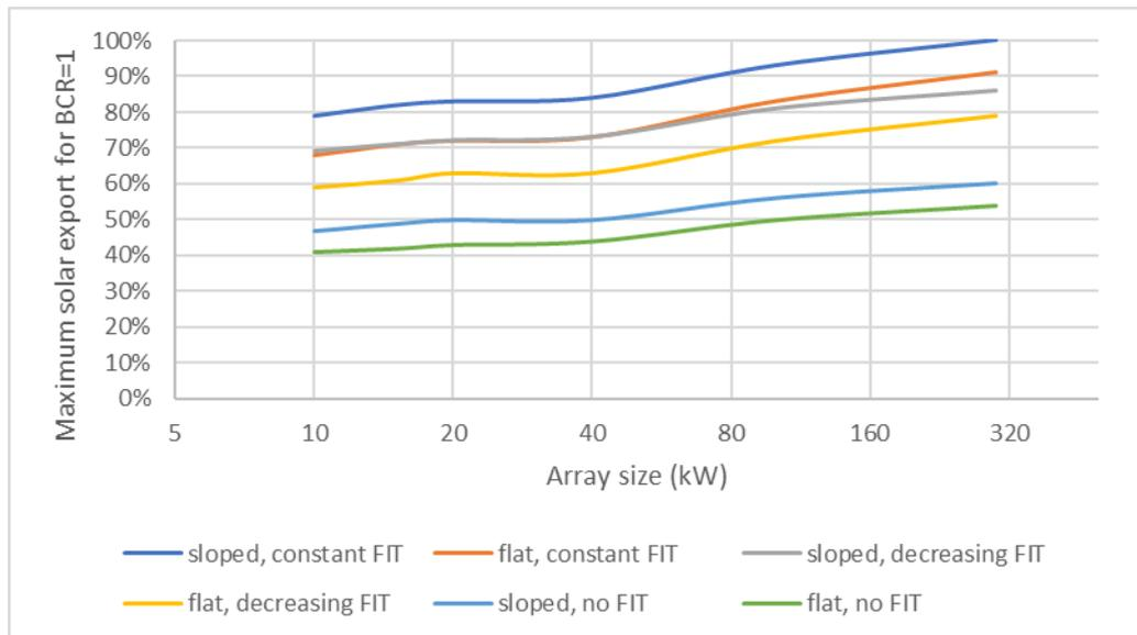
Figure 12. Maximum solar export from PV arrays for a benefit cost ratio of 1 under a range of Feed-in-tariff (FIT) scenarios, for sloped and flat installations.
