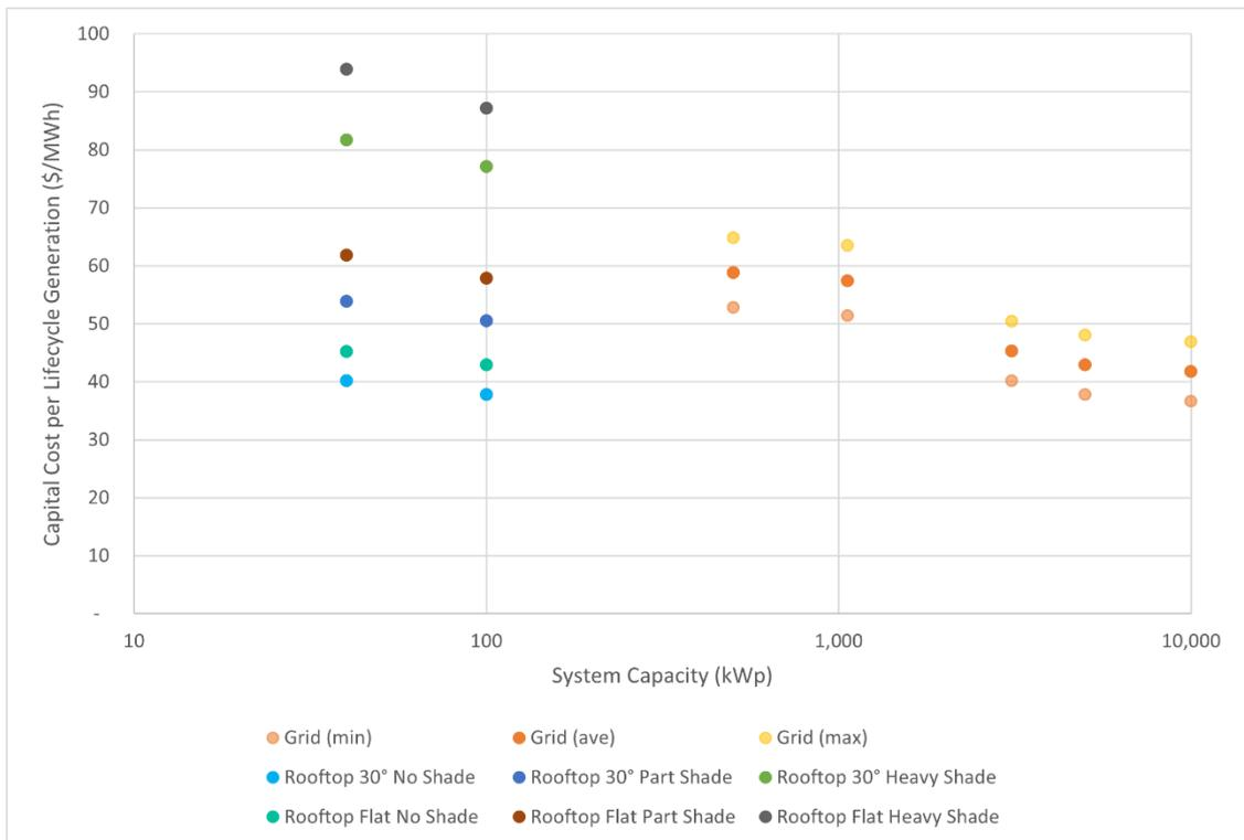
Figure 11: System Capital Cost per MWh of Lifecycle Generation for Rooftop and Grid PV
