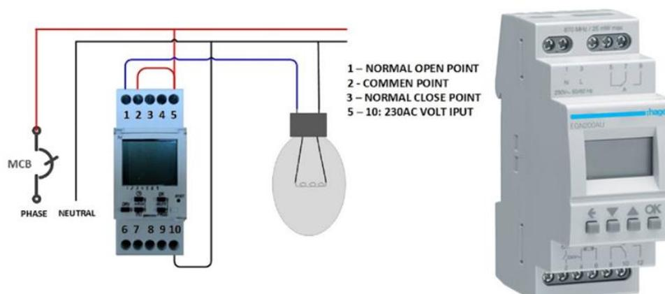
Figure 34: LCS-02 - Time switch operation
