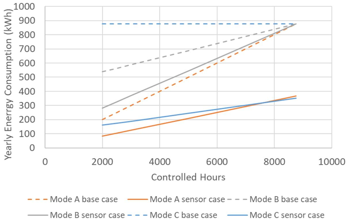
Figure 19. Comparison of energy use for Mode A, B and C cases of bathroom operation based on 100W load under sensor control. Note that in the Mode C base case, lights are always on.
