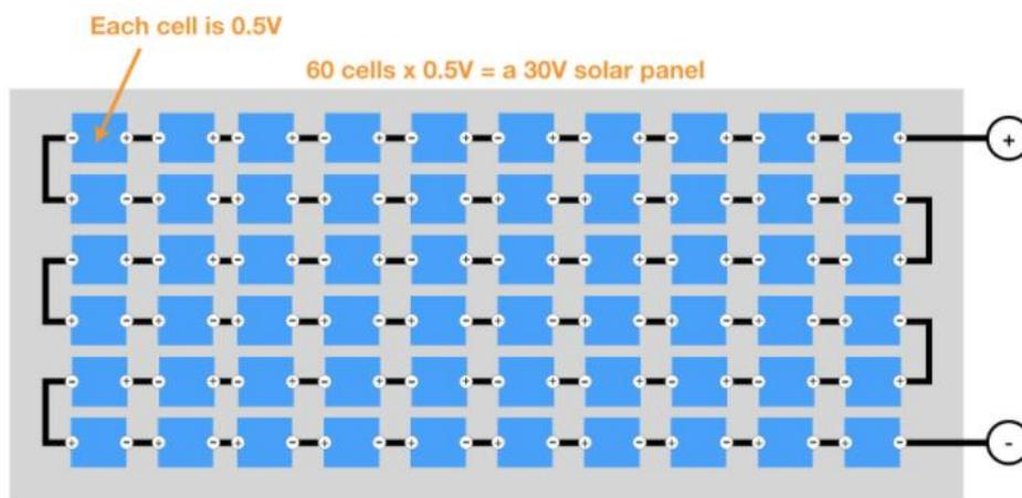
Figure 26: Conventional Solar PV Panel<sup>25</sup>
