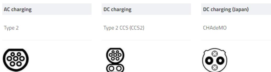
Figure 1: EV Charger Socket Outlet Types
