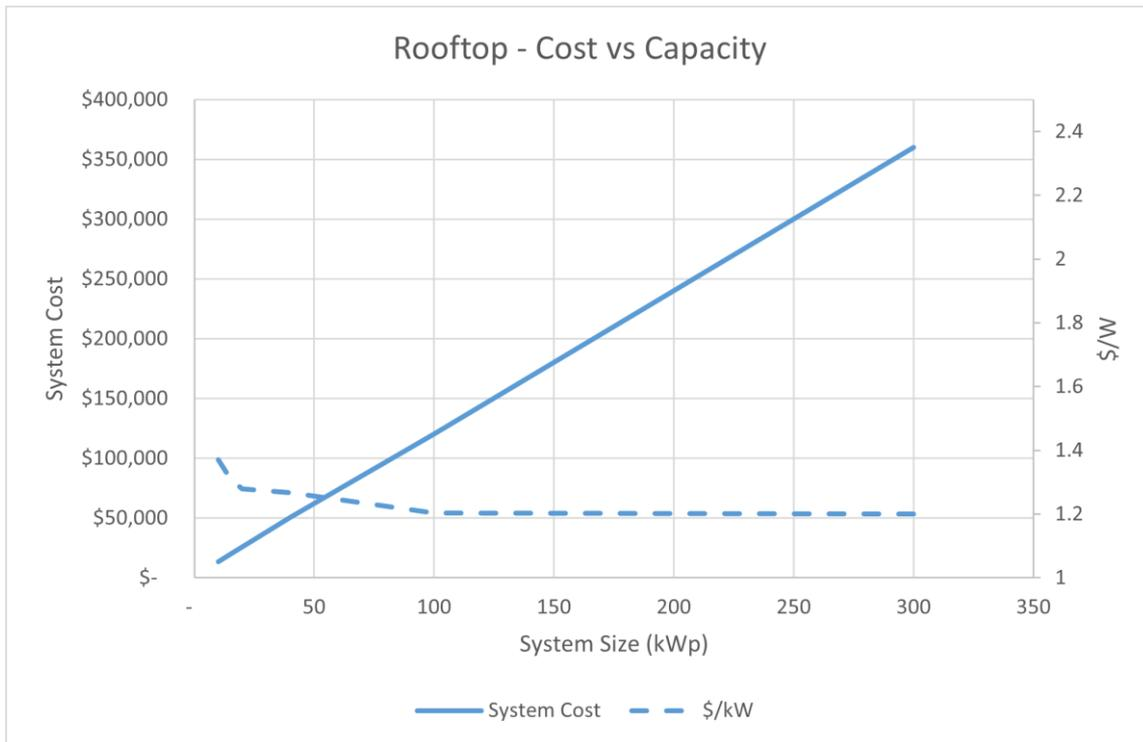
Figure 9: Cost vs Capacity for Rooftop Solar PV Installations
