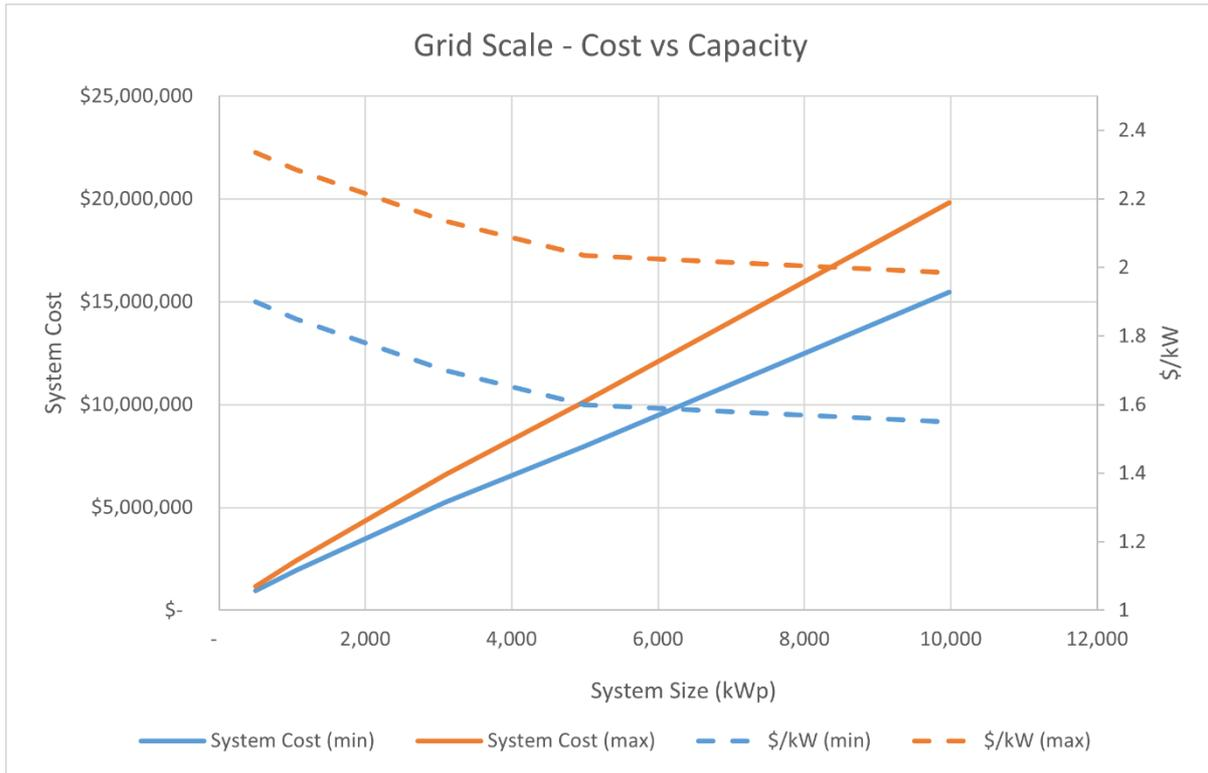
Figure 10: Cost vs Capacity for Grid Scale Solar PV systems
