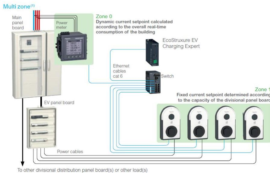
Figure 4: Active Load Management System<sup>2</sup>
