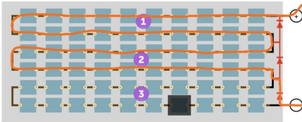
Figure 27: Conventional Solar PV Panel Shading Response<sup>26</sup>
