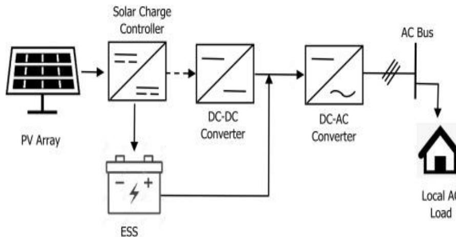
Figure 1: Solar PV system connected to load.<sup>24</sup>
