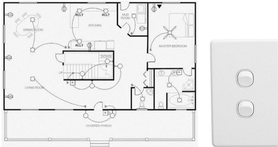
Figure 33: LCS-01 - Local Switching zones arrangement
