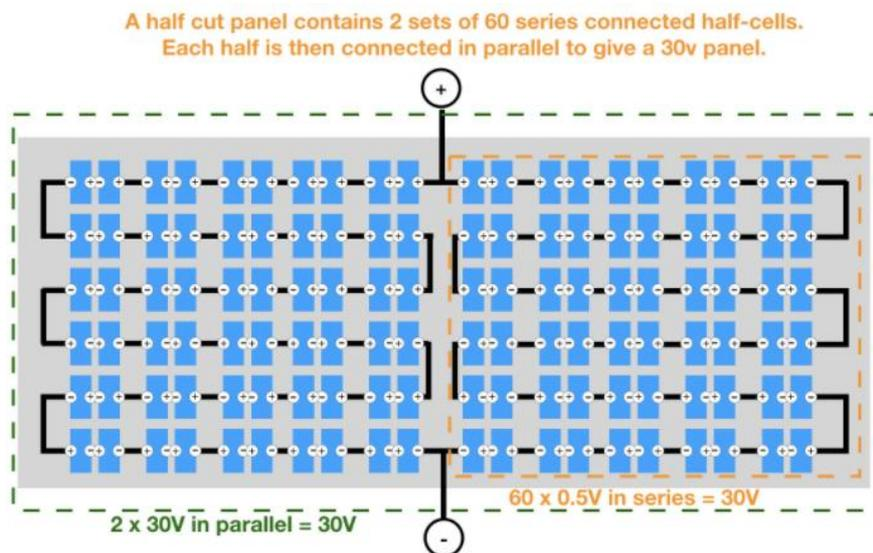
Figure 28: Half Cut Solar PV Panel<sup>27</sup>
