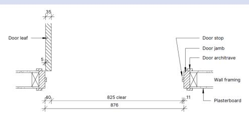
As illustrated, an 870 mm door would give us a total clearance of 825 mm, which exceeds the minimum clearance requirement of 820 mm. The Standard does not require the door handle to be considered for the minimum clearance.
