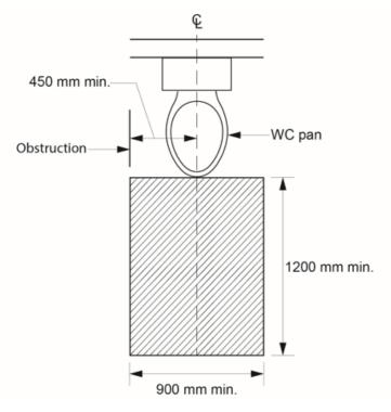
Where the toilet is located between opposing side walls, such as a typical stand-alone sanitary compartment, there must be a minimum of 900 mm between the finished wall surfaces. Where the toilet pan is within a room with other fixtures, the side of a vanity or other obstruction (e.g. bath) needs to be at least 450 mm from the centreline of the toilet pan. Figure 6.4 and Figure 6.5 illustrates different examples of the application of these requirements.
