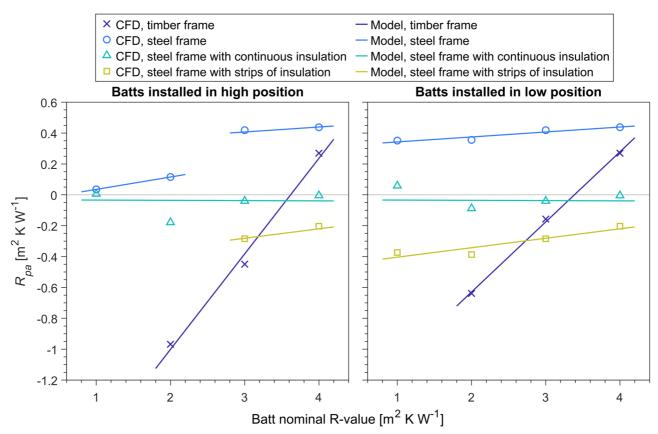
Figure 12: Models used to determine the pseudo air-space R-value,  $R_{pa}$ , which is used in the modified thermal bridge calculation method for suspended floors. Results obtained using these models are shown in Figure 11. Note that a separate model was developed for steel-framed floors that allow air exchange between the cavities inside each steel joist and the subfloor space (i.e. steel-framed floors with R1 or R2 insulation installed 'high' and no mitigation measures).
