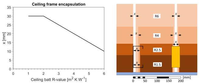
Figure 6: Levels of frame encapsulation modelled in cases with different ceiling batt R-values: (left) the function used to determine the gap between adjacent batts (x); and (right) cross-sections illustrating how batts of different R-values were assumed to fit around steel and timber frame members (note that the frame members are held 20 mm above the plasterboard by perpendicular battens, which are not intersected by these cross-sections).
