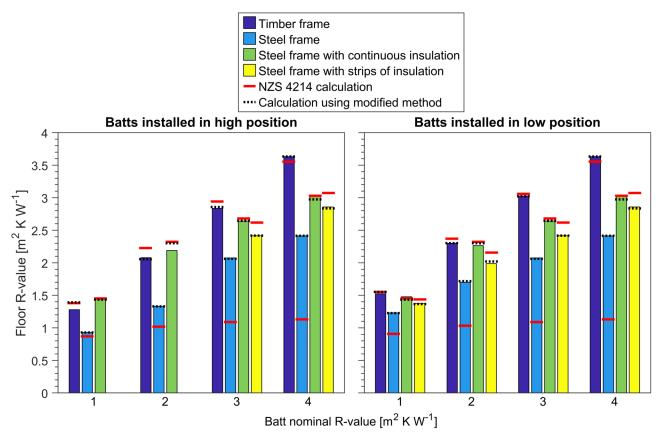
Figure 2: R-values of floor assemblies (not including 'film resistances') from CFD simulations of Cases 1–23, compared to standard NZS 4214 calculations and calculations using the modified method developed here. The left- and right-hand graphs display results from cases the bulk floor insulation is installed flush with the top and bottom surfaces of the floor joists, respectively. Results from cases where the bulk insulation height equals the joist height are included in both graphs.
