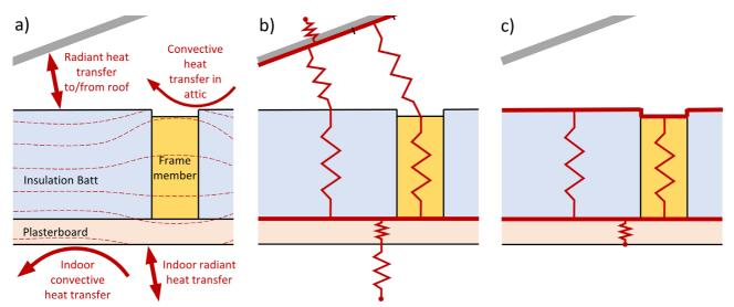
Figure 4: Schematic diagrams of heat transfer through a horizontal ceiling under a pitched roof: (a) primary heat transfer pathways and approximate isotherms (red dashed lines); (b) application of the NZS 4214 method to the entire ceiling and roof assembly; and (c) application of the NZS 4214 method to the ceiling assembly only (as required within the NCC).
