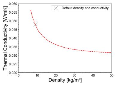
Figure 7: Variation of ceiling batt thermal conductivity with density, where the density increases in localised regions of batt compression above ceiling battens. The function in this table is based on material data published in the AIRAH Technical Handbook [15].
