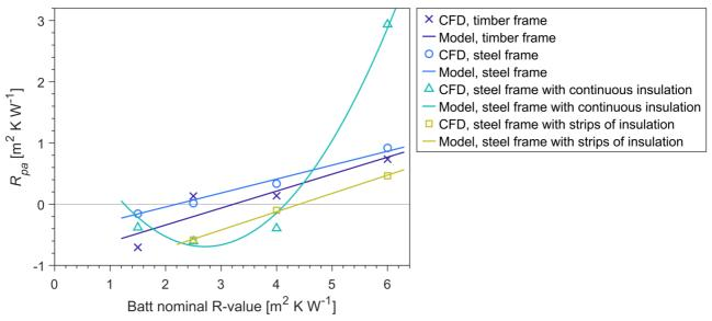
Figure 9: Models used to determine the pseudo air-space R-value,  $R_{pa}$ , which is used in the modified thermal bridge calculation method for ceilings. Results obtained using the method are shown in Figure 8.
