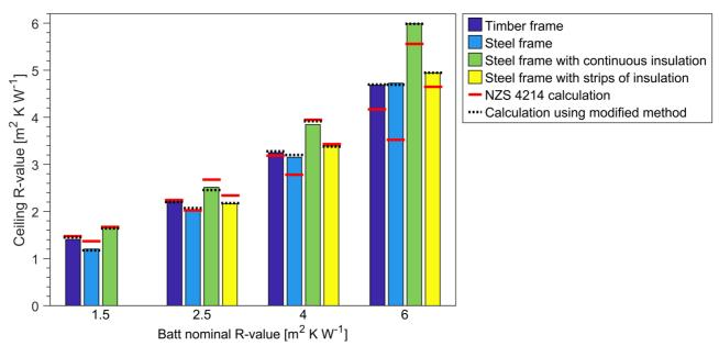
Figure 8: Ceiling R-values (not including 'film resistances') determined from CFD simulations of Cases 1–15, and compared to values calculated using: (i) the NZS 4214 method, and (ii) a modified method developed in this study and calibrated using the CFD results.
