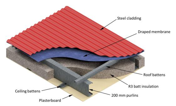
Figure 13: Partial cut-away diagram showing a section of the skillion roof design that was analysed.
