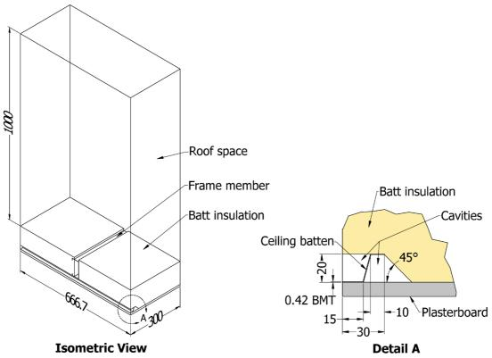
Figure 5: Example of the type of three-dimensional computational domain developed for the simulations of horizontal ceilings under pitched roofs. Only half of the batten was included in the domain, and a 'symmetry' boundary condition was applied to the plane that cuts the batten in half. Dimensions are expressed in mm.
