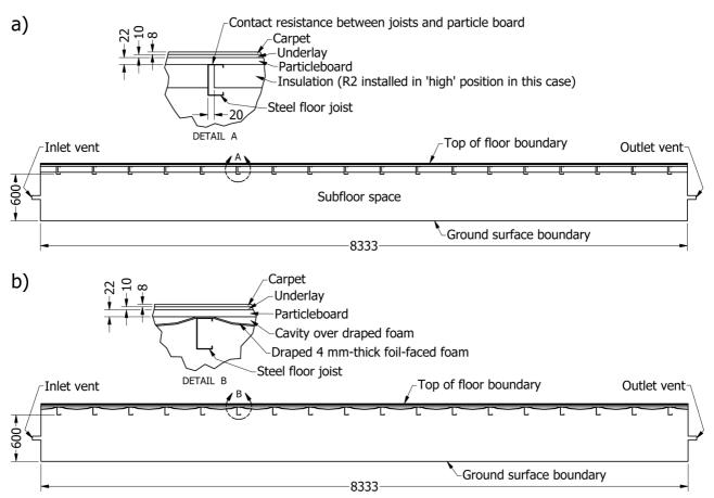
Figure 10: Computational domains used to simulate a suspended floor and subfloor spaces including (a) Case 3, with bulk insulation installed between joists; and (b) Case 27, with draped foil-faced foam insulation. All dimensions are expressed in mm.
