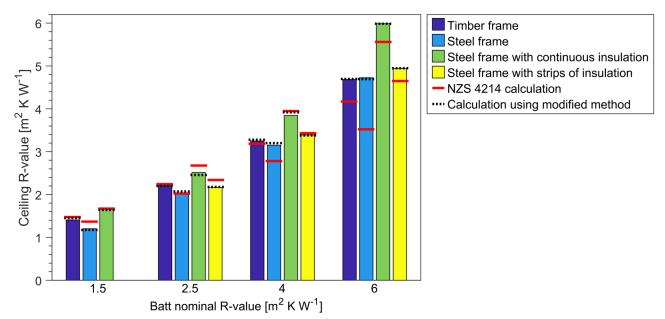
Figure 1: Ceiling R-values (not including 'film resistances') determined from CFD simulations of Cases 1–15, and compared to values calculated using the NZS 4214 method and a modified method developed in this study and calibrated using the CFD results.
