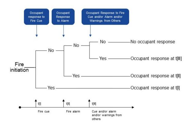
Each of the above four occupant detection response scenarios, as shown in Figure 3.1.3, should be combined separately with each of the fire scenarios identified in Figure 3.1.2.
