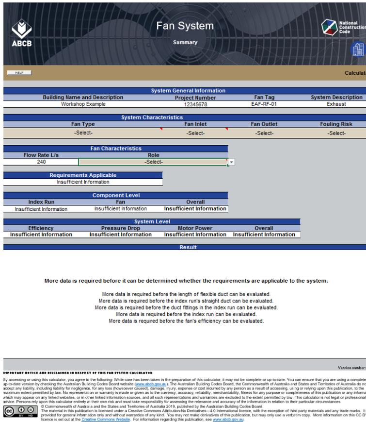
The following is a description of the format and key cells in the Fan System Calculator to explain its use. Additional advice can be found in the Help Screen of the Calculator.
