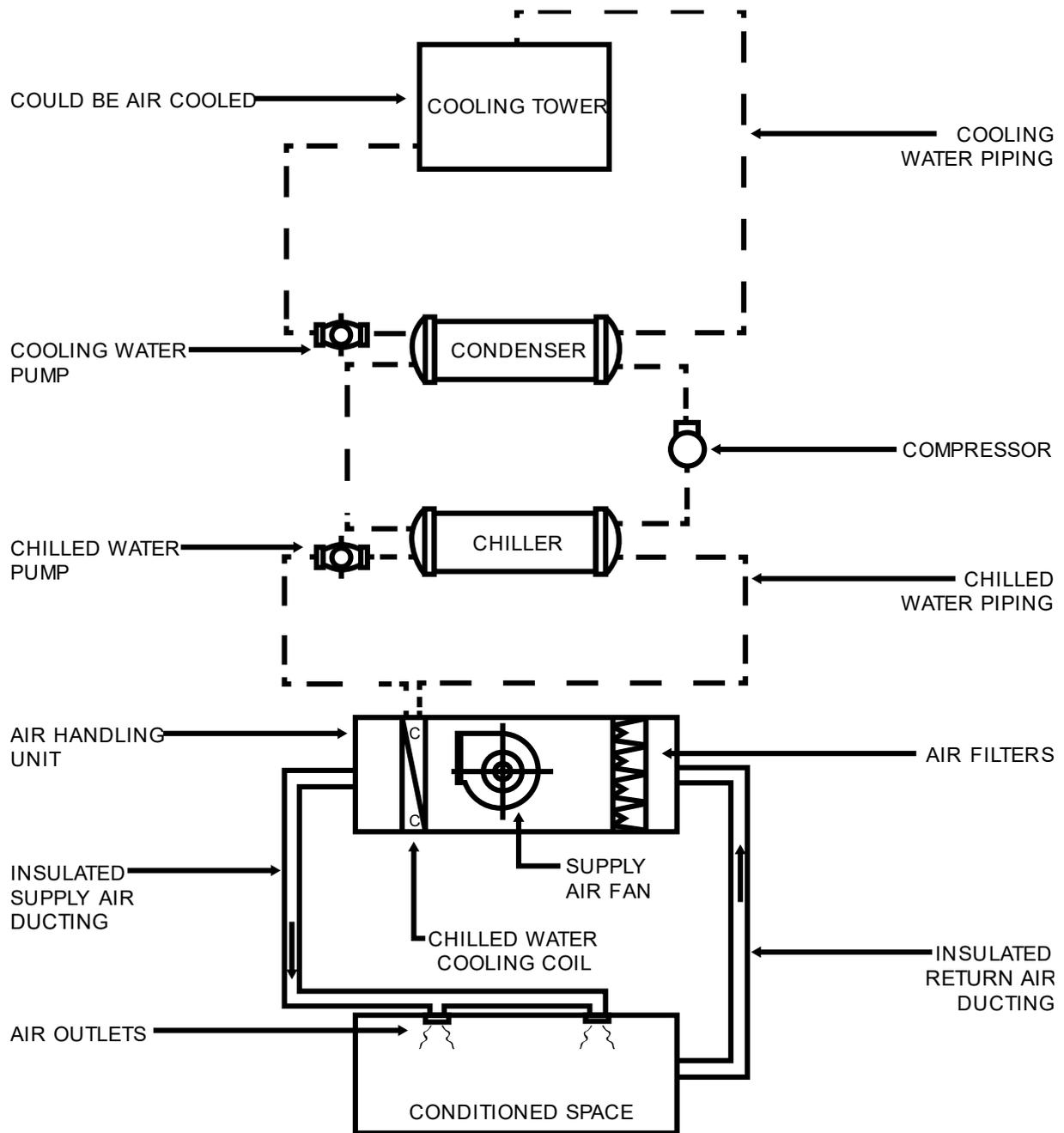
The *AHU* can be a central system serving more than one area and/or multiple floors, or alternatively, an individual *fan coil unit (FCU)* can be provided for each individual space. For further information, refer to the explanation of *AHU* and *FCU*.
