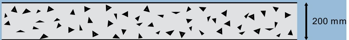
A solid concrete slab is 200 mm thick.
