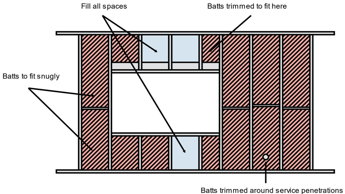
The requirement recognises that the practical limitations of maintaining the position and thickness of bulk insulation where it is likely to be compressed between cladding, supporting members, water pipes and electrical cabling. In these instances, compression of the bulk insulation may occur but should be limited where possible.
