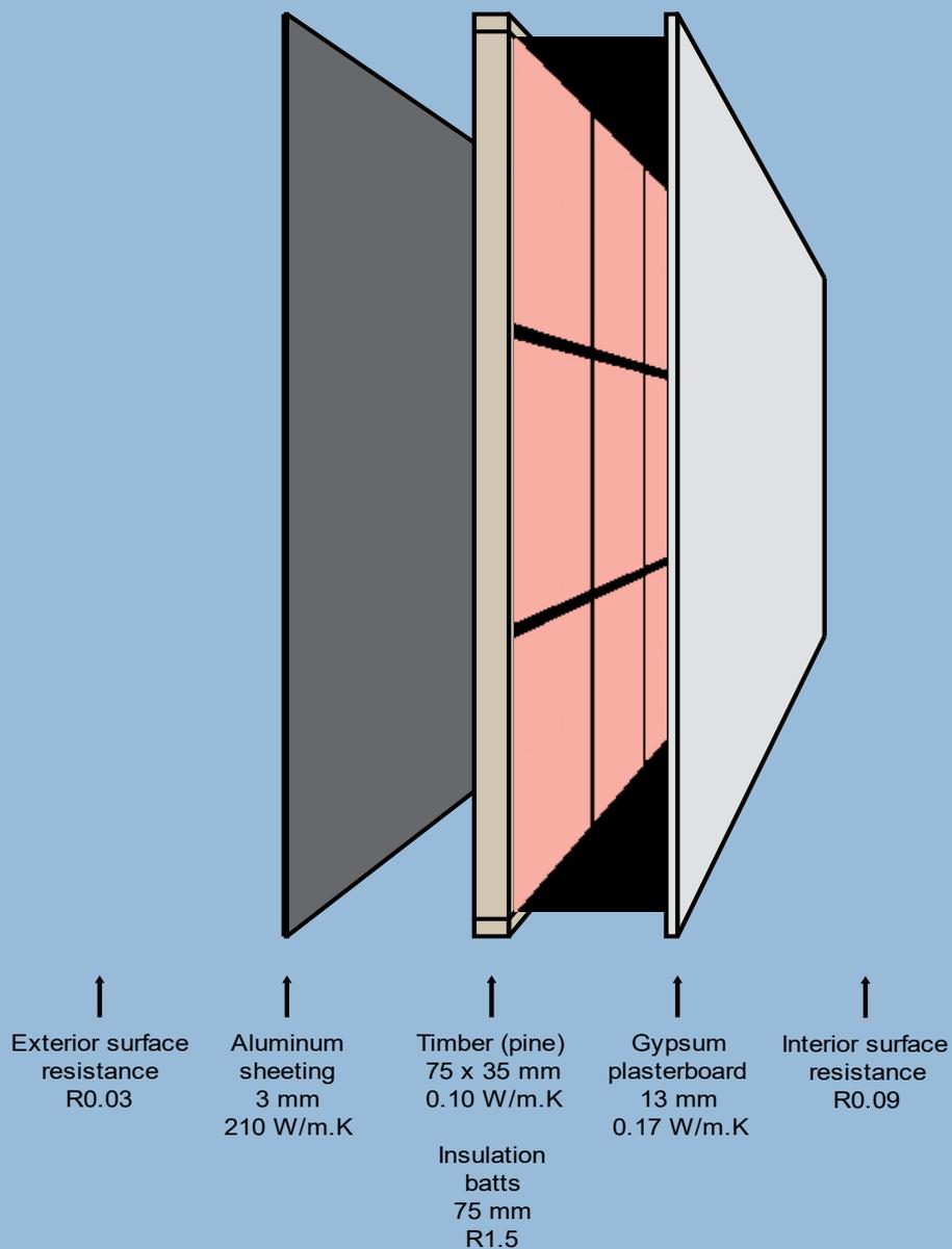
The *Total R-Value* is calculated by determining the thermal resistance of each layer, surface layer, and any bridged layers in the wall.
