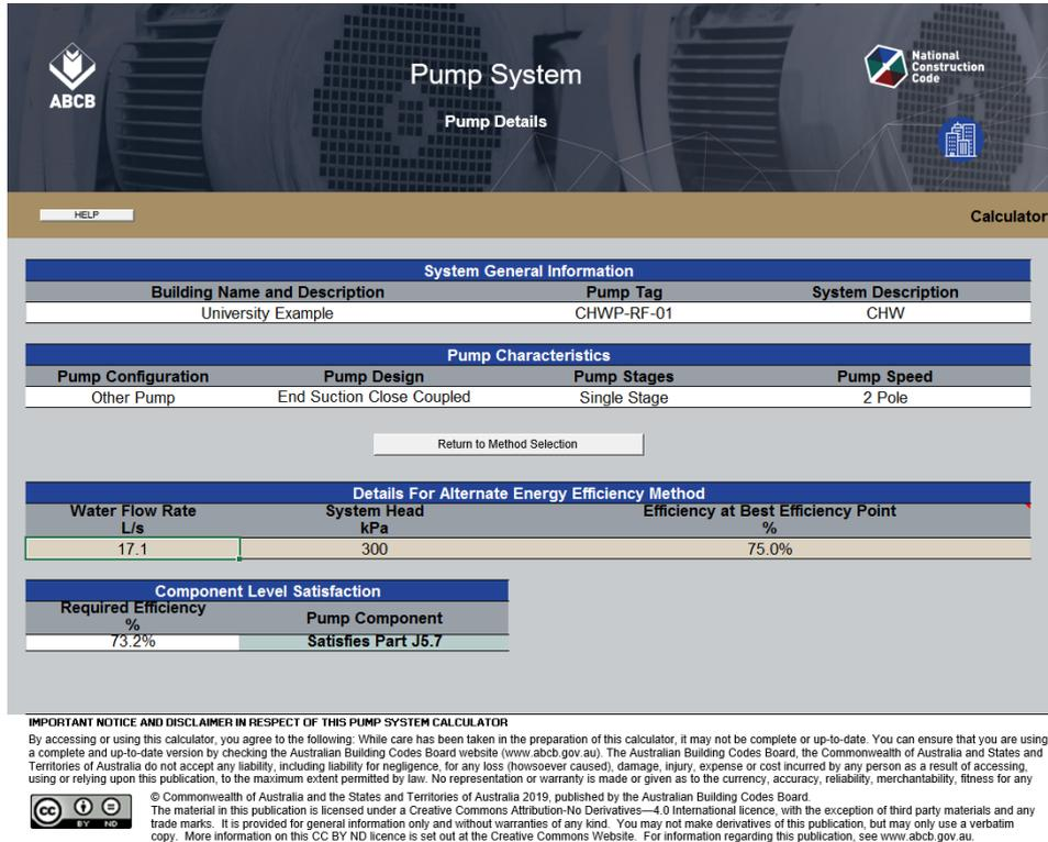
Figure 13.21 shows the Pump System Calculator evaluating the pump compliance using the Alternate Method for Pump Details. The Alternate Method requires more information than the Simple Method, however it can analyse the system, for compliance with either J5.7(a)(i) or J5.7(a)(ii).
