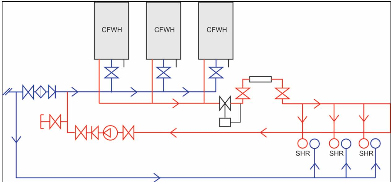
Figure 8: Typical example of a single pipe warm water circulating system controlled by a bank of continuous flow water heaters.
