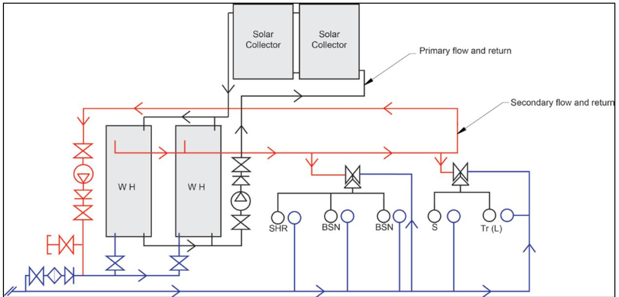
**Figure 10: Typical example of a primary flow and return solar system.**
