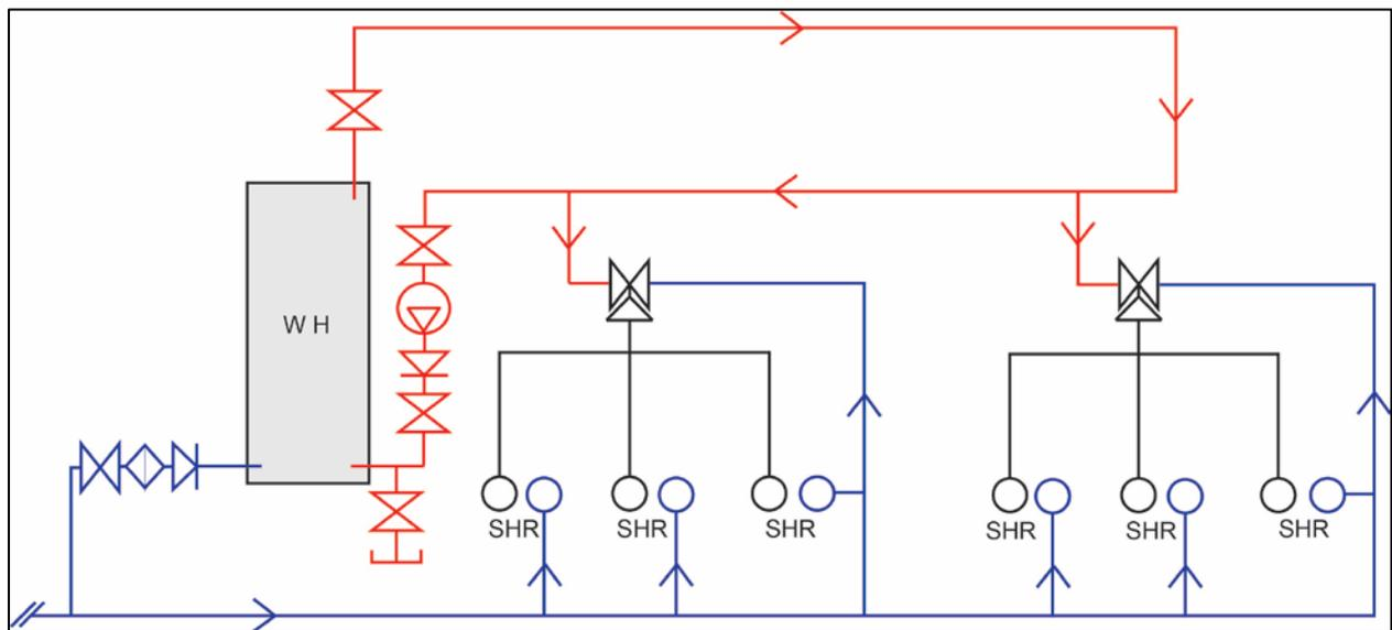
Figure 7: Typical example of a single pipe circulating system.
