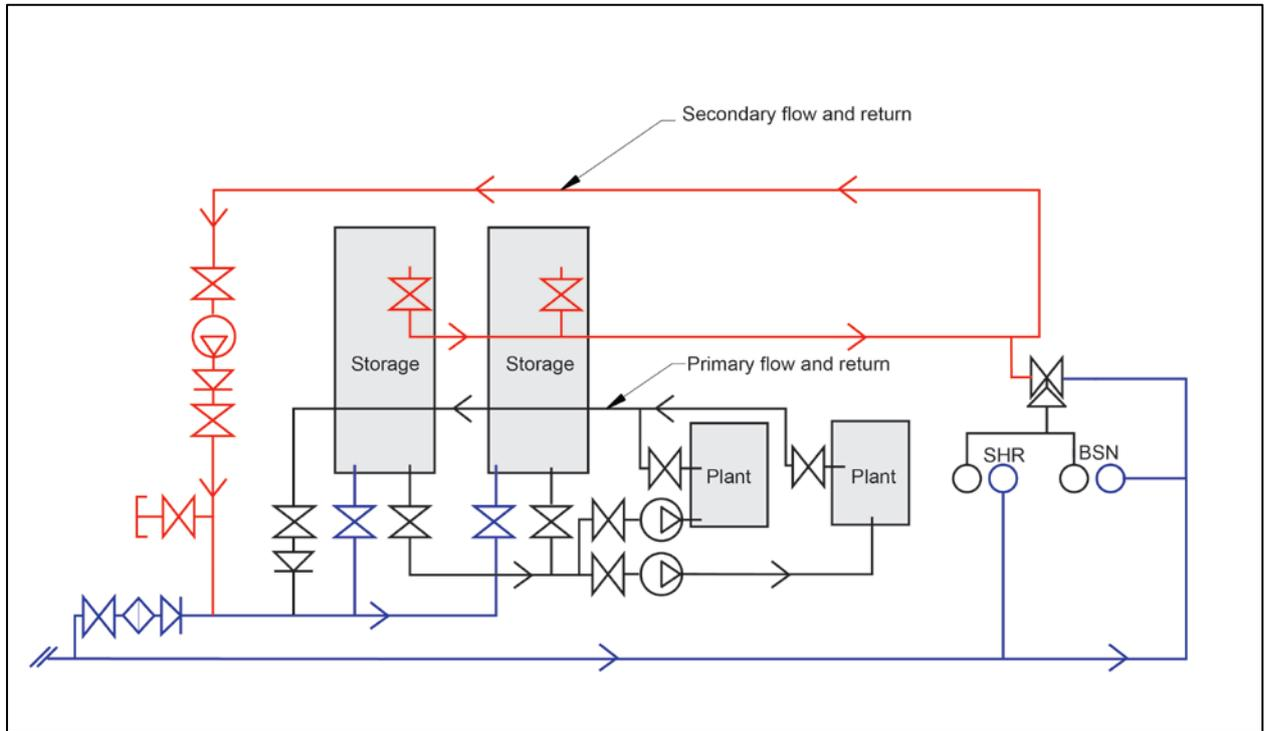
Figure 12: Typical example of a primary flow and return system through heating plant.
