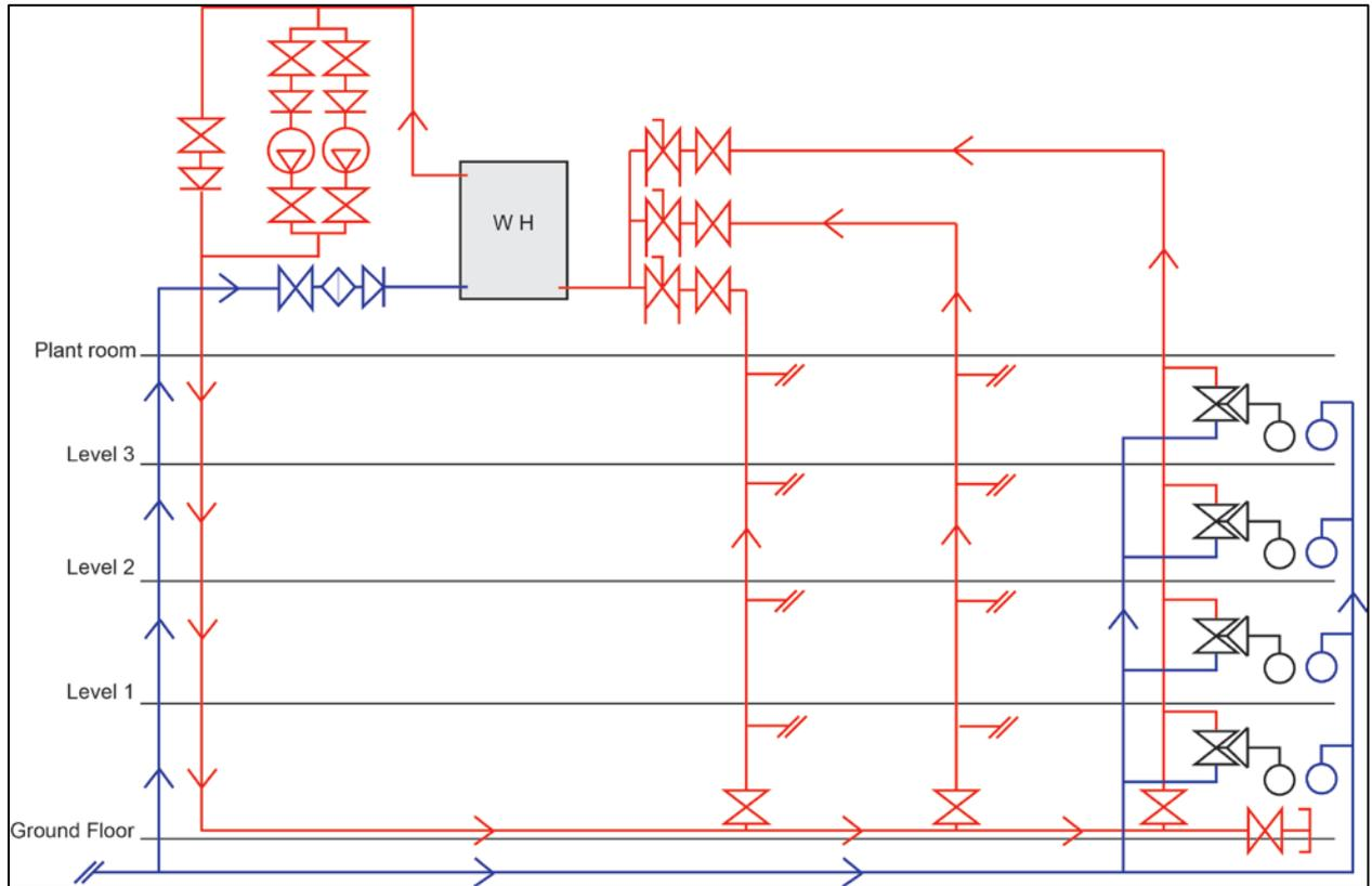
Figure 14: Typical example of heated water flow and return system with pumps on flow line.
