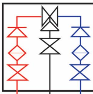
Figure 18: Integral components of a thermostatic mixing valve
