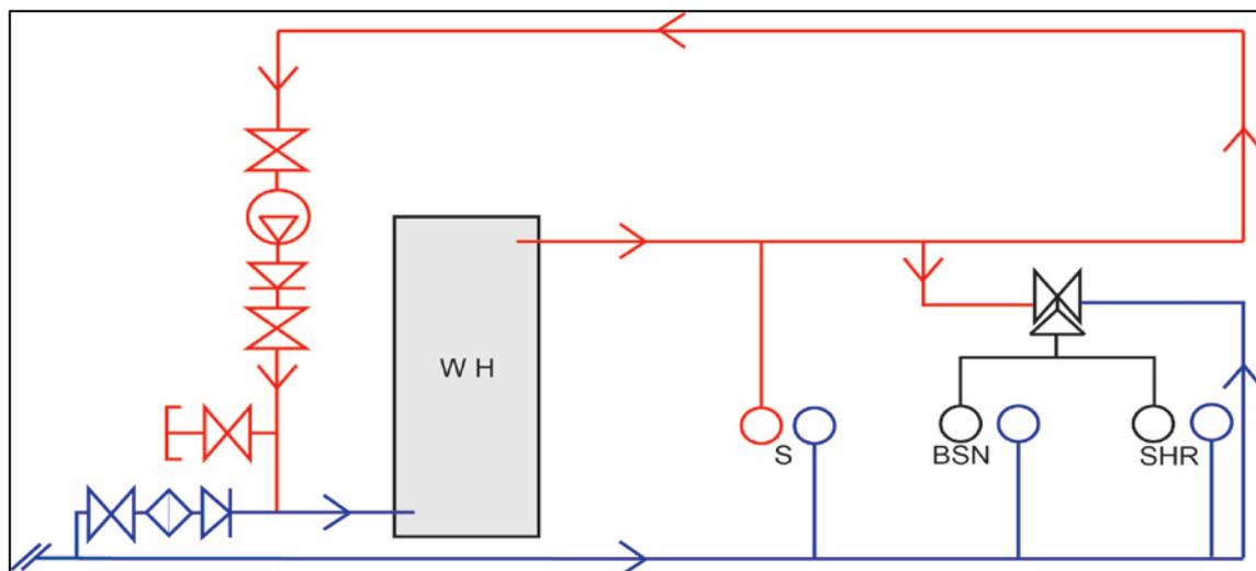
Figure 4: Typical example of a circulating warm water system controlled by a TMV.
