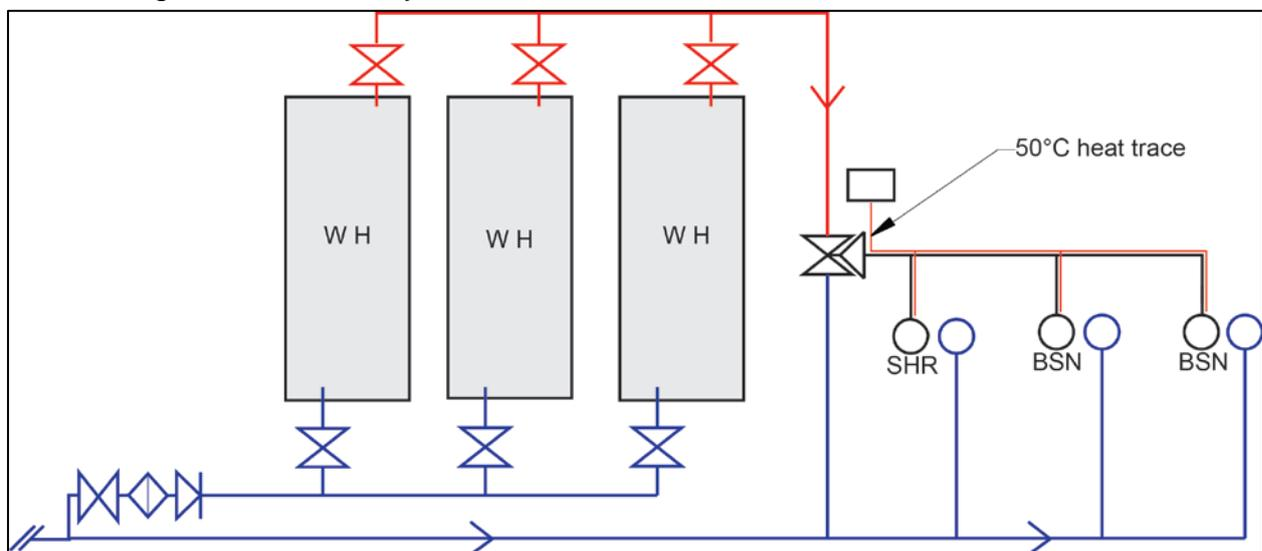
**Figure 3: Typical example of a reticulated warm water system incorporating heat trace wire.**
