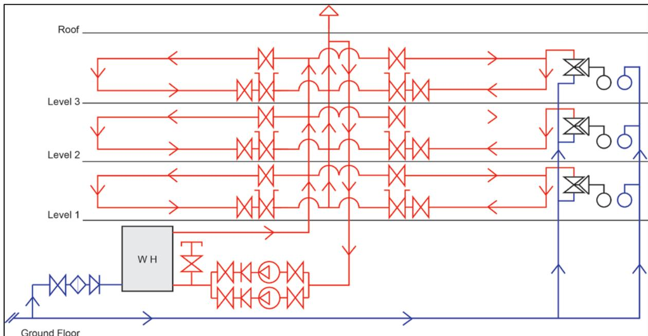
Figure 15: Typical example of a two pipe – Direct return system.
