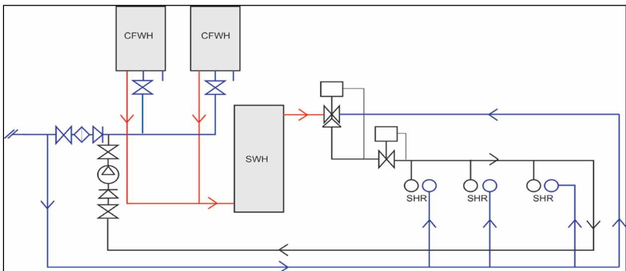
**Figure 6: Typical example of a circulating warm water system controlled by a modulation valve with a temperature sensor.**
