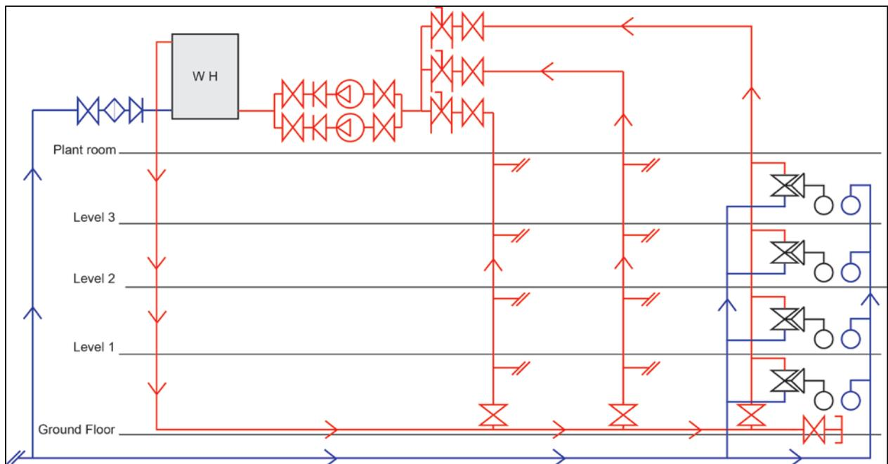
Figure 13: Typical example of heated water flow and return system with pumps on return line
