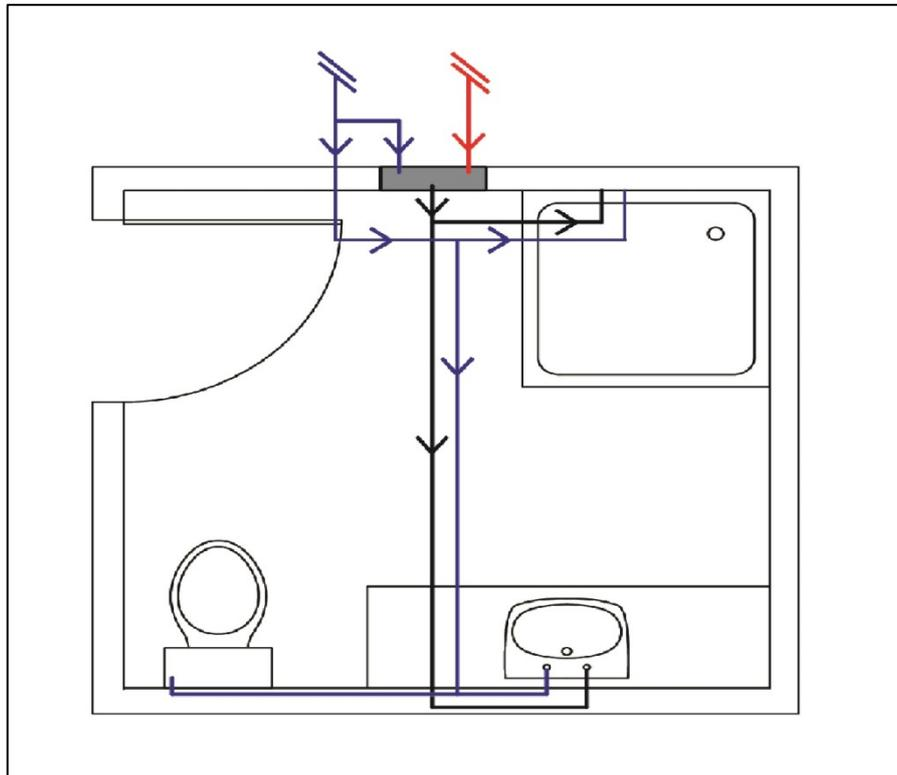
**Figure 17: Typical bathroom pipework layout**
