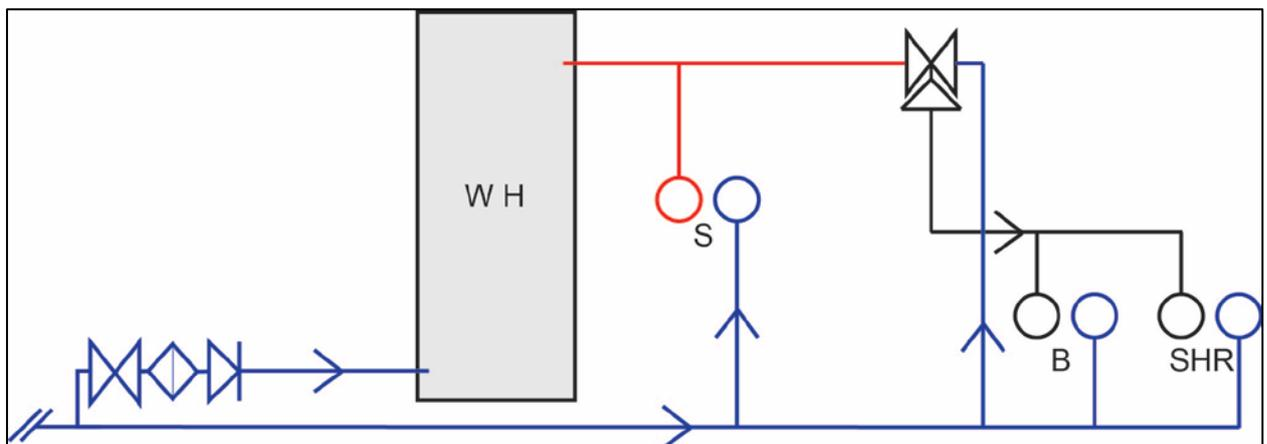
Figure 2: Typical example of a partially tempered reticulated warm water system.
