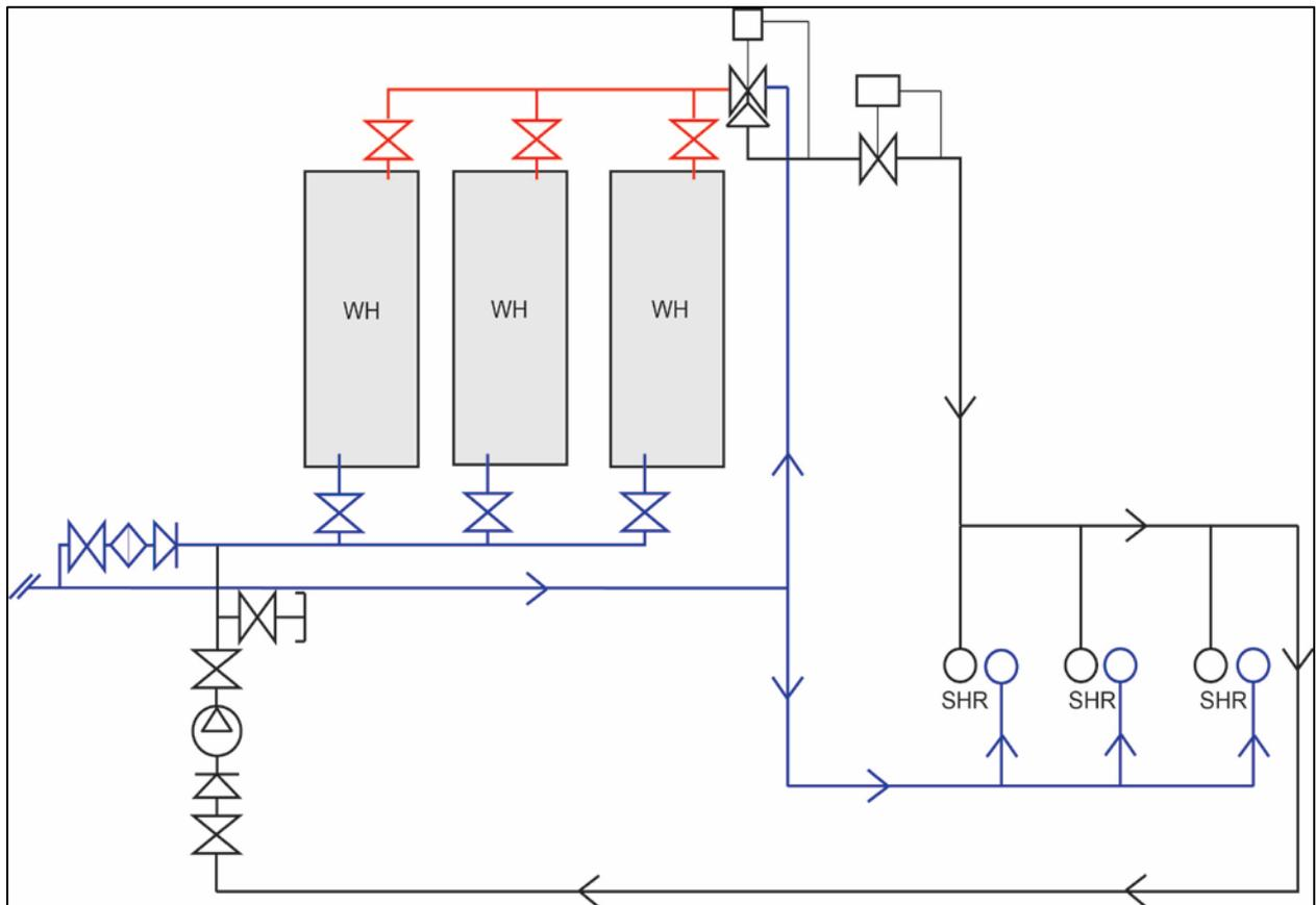
Figure 9: Typical example of a single pipe warm water circulating system controlled by a modulating valve through a bank of water heaters.
